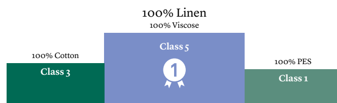
Moisture Management Tester classification scale 1 to 6 - AATCC 195 standard
